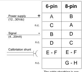
The cable sheathing is connected to the transducer body
